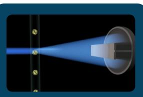
During flow cytometry, a laser strikes MPs and EPCs, sending scattered light data to a detector.
